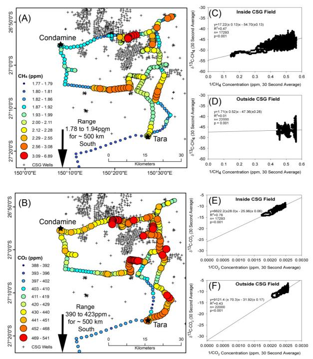
Figure 1: Spatial survey in the Tara region. (A).  $CH_4$  concentrations, (B)  $CO_2$  concentrations, (C) Keeling plot of  $CH_4$  within the gas field, (D) Keeling plot of  $CH_4$  outside of the gas field, (E) Keeling plot of  $CO_2$  within the gas field, (F) Keeling plot of  $CO_2$  outside of the gas field. The crosses indicate the location of CSG wells.
