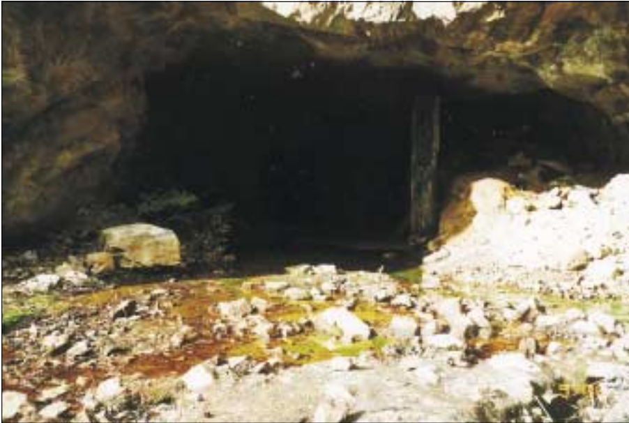
Plate 10. Acid drainage discharge from Round Hill adit, Sheffield area
