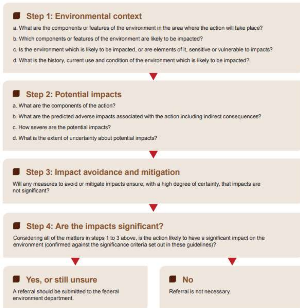
Figure 102 - Diagram summarising the self-assessment process. Source: Department of the Environment and Energy, https://www.environment.gov.au
