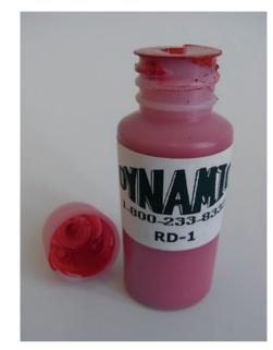
Figure 1 Example of inadequate sealing of a tattoo ink stock bottle at receipt by customer. Broken membrane with leakage of red tattoo ink.
