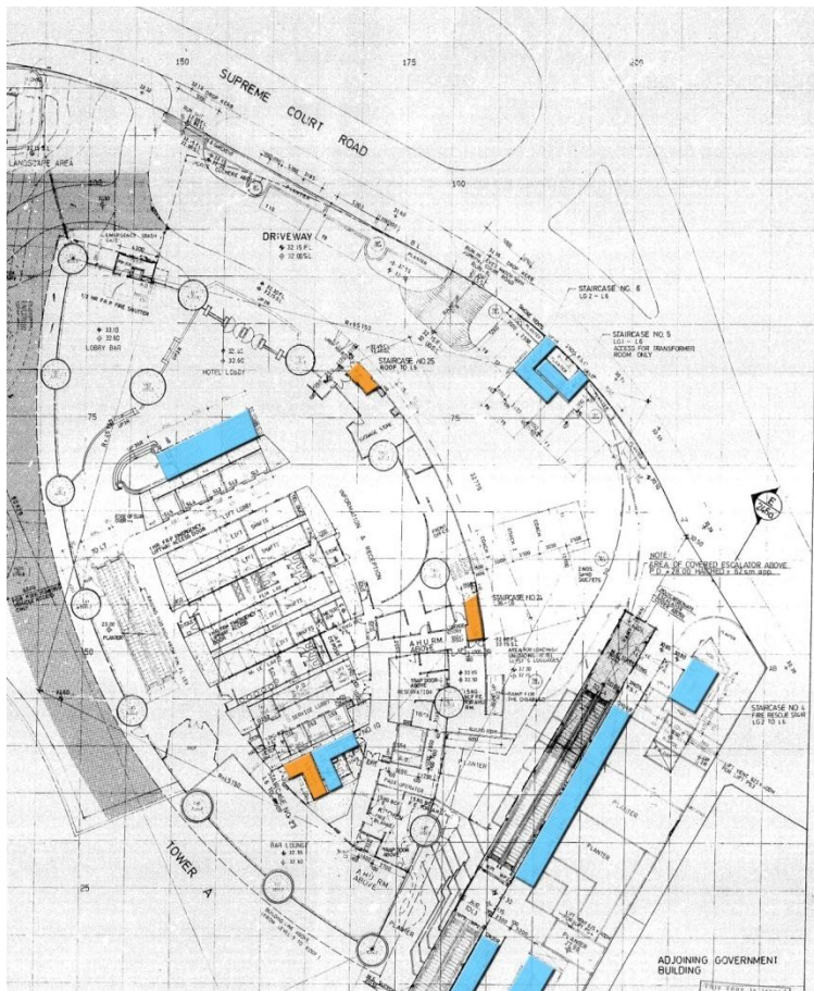
Figure 29: Ground (level 6), orange stairs are ascending and blue stairs are descending (Wong & Ouyang 1991b)
