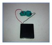
2. Push the lumps together so they touch and the LED turns off. This happens because electricity flows through the conducting dough more easily than through the LED. This is called a short circuit.
