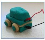
Once your circuit is working, add more play dough to make any shape you like. Just remember to keep the conducting parts of the sandwich apart.
