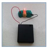
3. Use a small lump of the non-conducting dough to separate the two lumps. The LED lights up again even though all the lumps are touching. Electricity does not flow through the non-conducting dough very easily.
