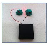
1. Make two small lumps of conducting dough. Poke one of the battery wires into each lump. Bend the LED legs and poke one into each lump (turn the LED around if it doesn't light up).
