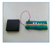
4. To light up more LEDs, make two long worms of conducting dough. Put a long worm of non-conducting dough between them. Poke one wire into each of the conducting dough worms. Now poke in as many LEDs as you like. This is called a parallel circuit.
