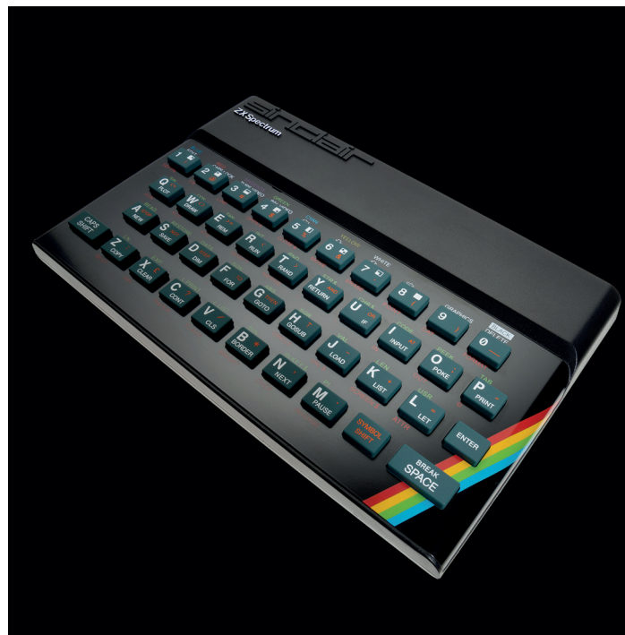
The chips are down: the original 48K Sinclair Spectrum: writing for its 1-bit beeper, Matt Rogers says, 'is as much a feat of programming as it is of composition
